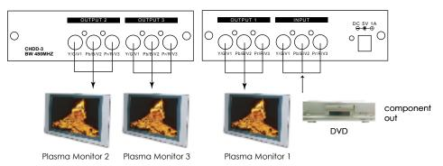
Works as a 1-in 3-out distribution amplifier for HD RGsB (Sync on Green) video source.
