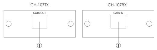
① CAT6 OUT/IN: Connect the CAT6 output of the transmitter with a CAT6 cable to the CAT6 input of the receiver.
